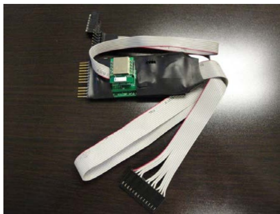
Credit and ATM card skimming device found inside a gas station pump
